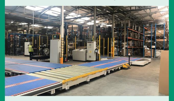
During June and July this year we've made some big changes to the factory at our Milton Keynes site! We've installed brand new conveyors for a fully-automated line able to handle products up to 3m wide, with barcode readers to accurately monitor all our stock, and an inline pallet press and stretch wrapper.
